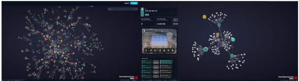
Figure 3: Comprehensive Semantic Model and Partial View of the Chiller System with Integration with BIM
