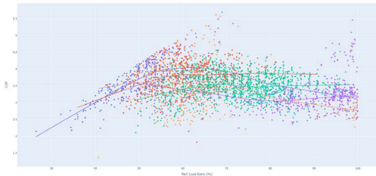
Figure 6: Chiller Performance Curve against Part Load Ratio under Different Wet Bulb Temperature Range
